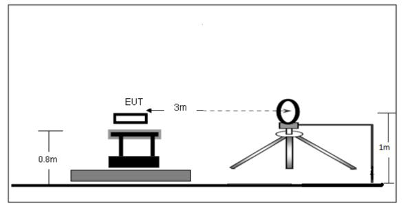
(B) Radiated Emission Test-Up Frequency 30MHz~1GHz
