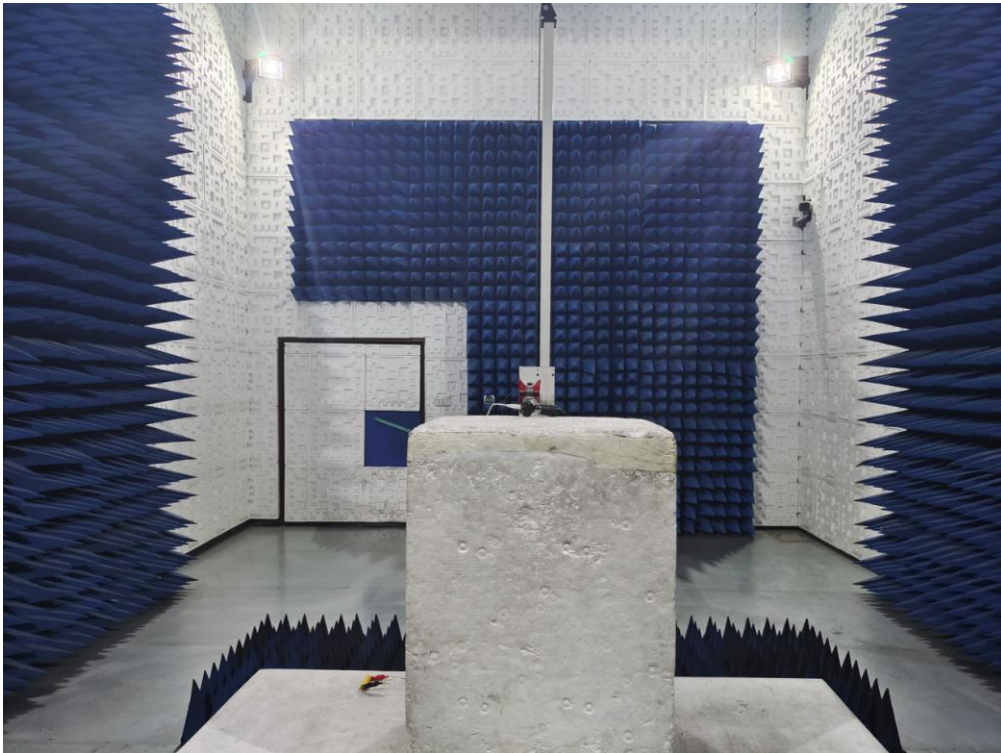
RADIATED EMISSION TEST SETUP ABOVE 1GHz
