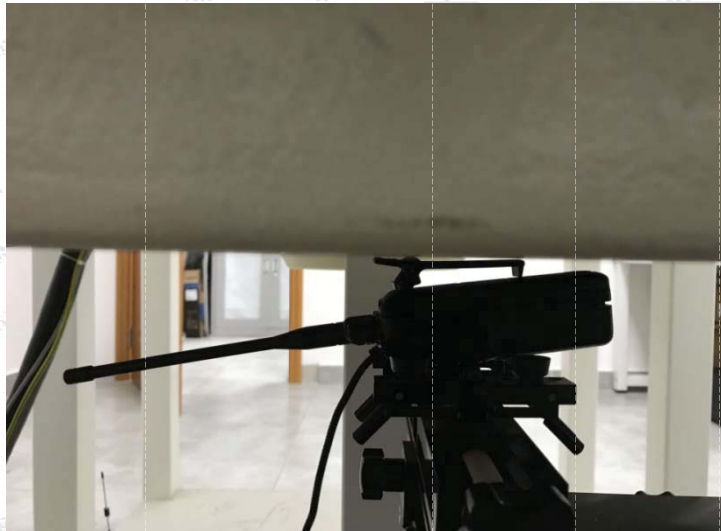
Body-worn, the front of the EUT towards ground with A1, B2 and D1 (The distance was 0mm)
