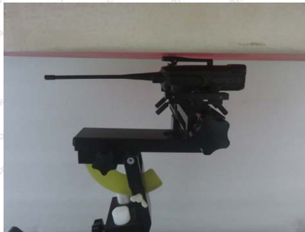
Body-worn, the front of the EUT towards ground with A1, B2 and D1 (The distance was 0mm)
