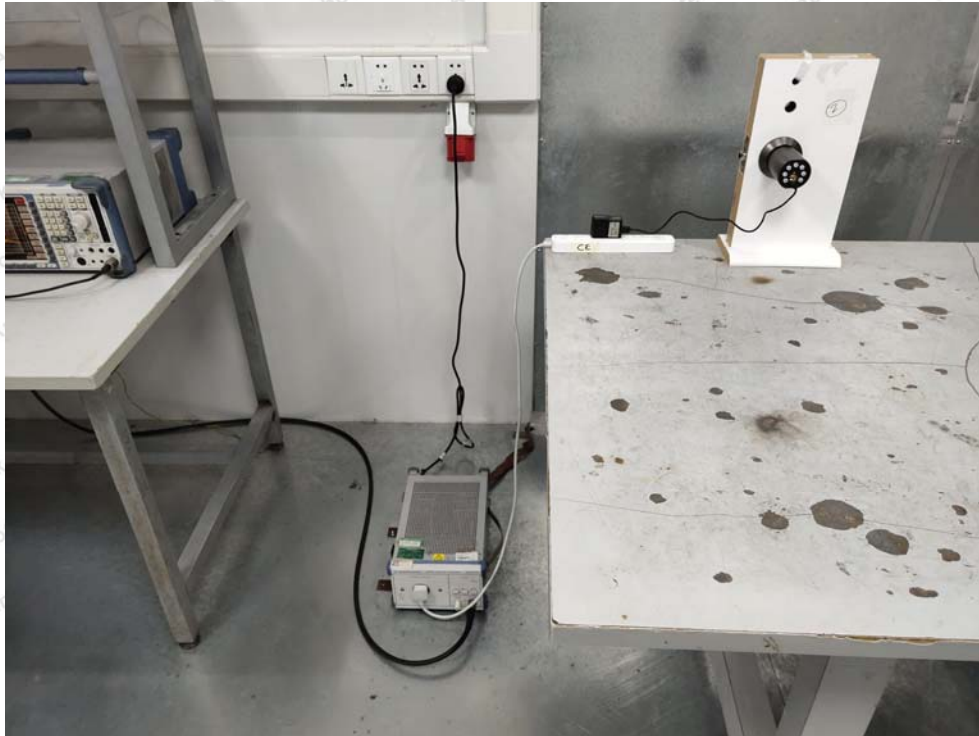
Photo of Power Line Conducted Emission Test
