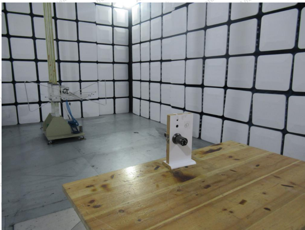
Photo of Radiation Emission Test
