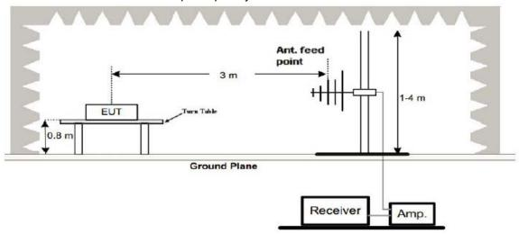
(3) Radiated Emission Test-Up Frequency Above 1GHz
