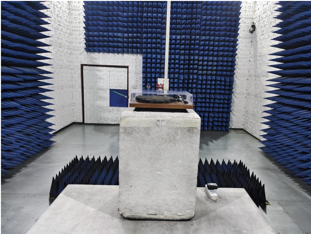
RADIATED EMISSION TEST SETUP ABOVE 1GHz
