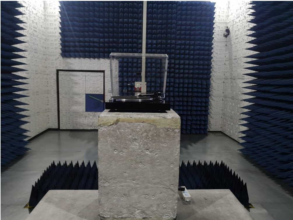
RADIATED EMISSION TEST SETUP ABOVE 1GHz
