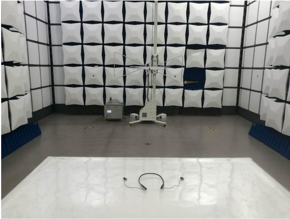
FCC RADIATED EMISSION TEST SETUP
