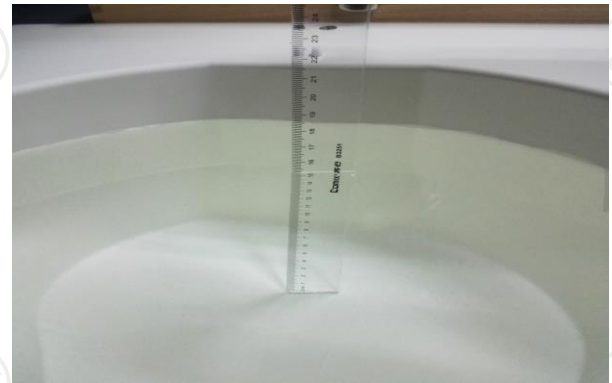
The Body Liquid of 2450MHz (15.3cm)
