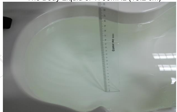
The Head Liquid of 2450MHz (15.6cm)
