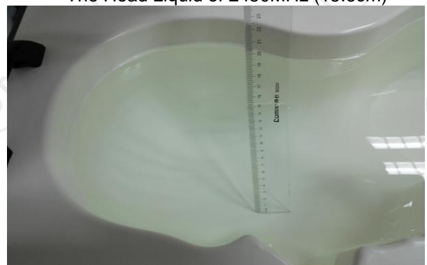
The Head Liquid of 1700MHz (15.2cm)
