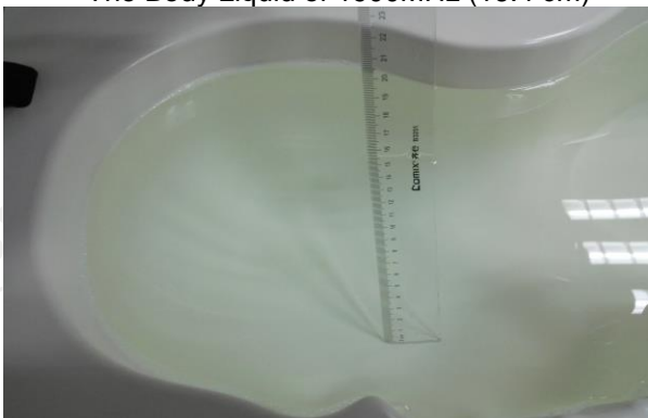
The Head Liquid of 1900MHz (15.5cm)
