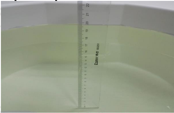
The Body Liquid of 835MHz (15.4cm)
