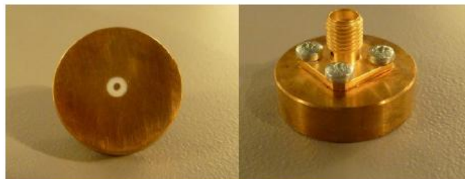
Figure 1 – MVG LIMESAR Dielectric Probe
