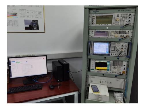
**RF** radiated test setup
