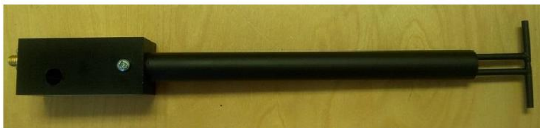
Figure 1 – MVG COMOSAR Validation Dipole
