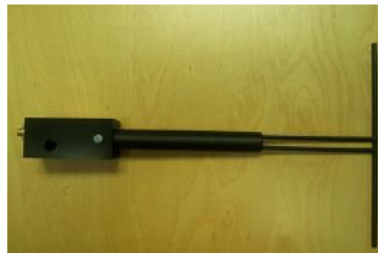
Figure 1 – MVG COMOSAR Validation Dipole
