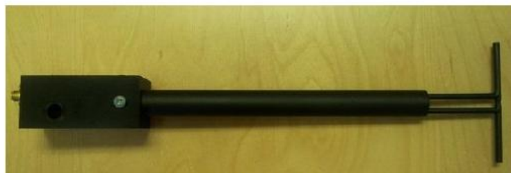
Figure 1 – MVG COMOSAR Validation Dipole
