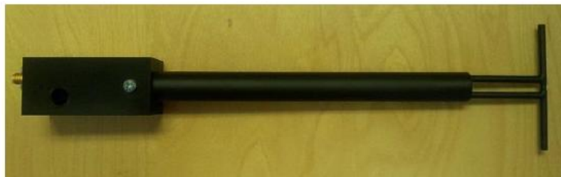
Figure 1 – MVG COMOSAR Validation Dipole
