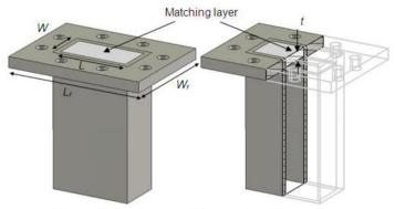
Figure 1: Validation Waveguide Dimensions
