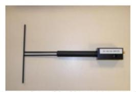
Figure 1 – Satimo COMOSAR Validation Dipole
