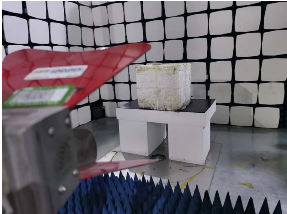
Radiation Emission Test Setup (1GHz to 18GHz)
