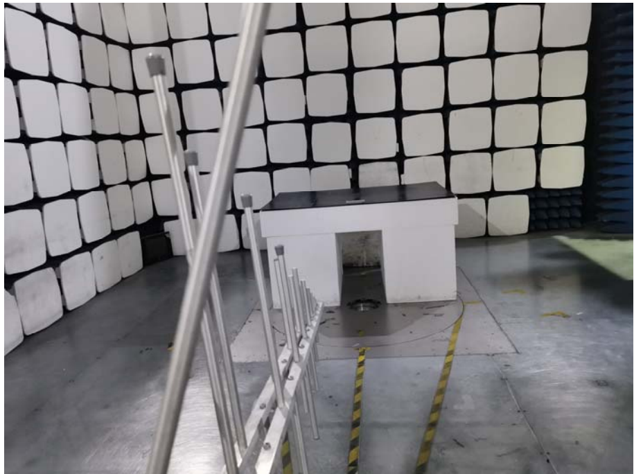
Radiation Emission Test Setup (30MHz to 1GHz)
