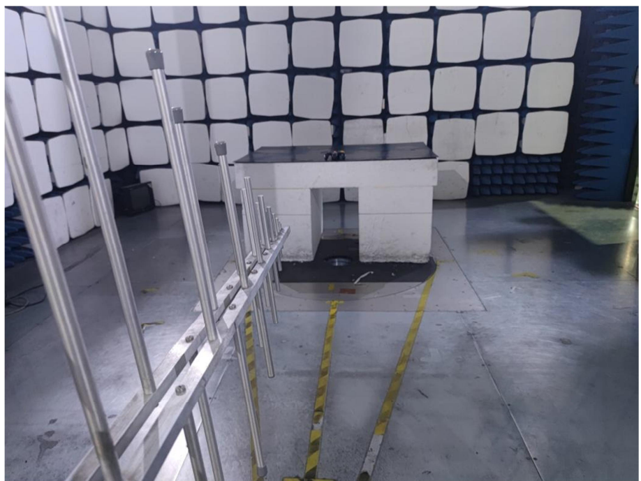
Radiation Emission Test Setup (30MHz to 1GHz)
