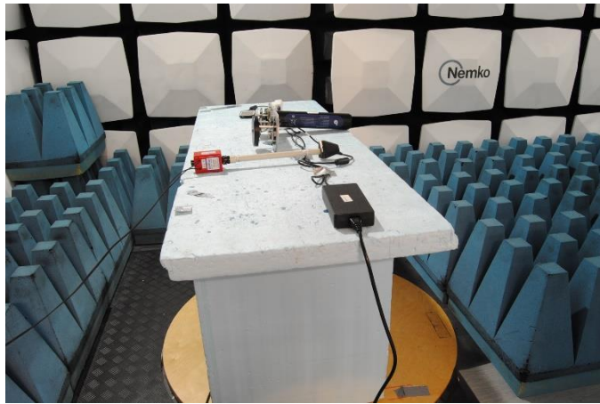
Test set-up for EMC immunity tests
