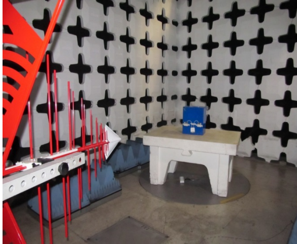
Radiated emissions test set up in 30MHz-1GHz freq. range
