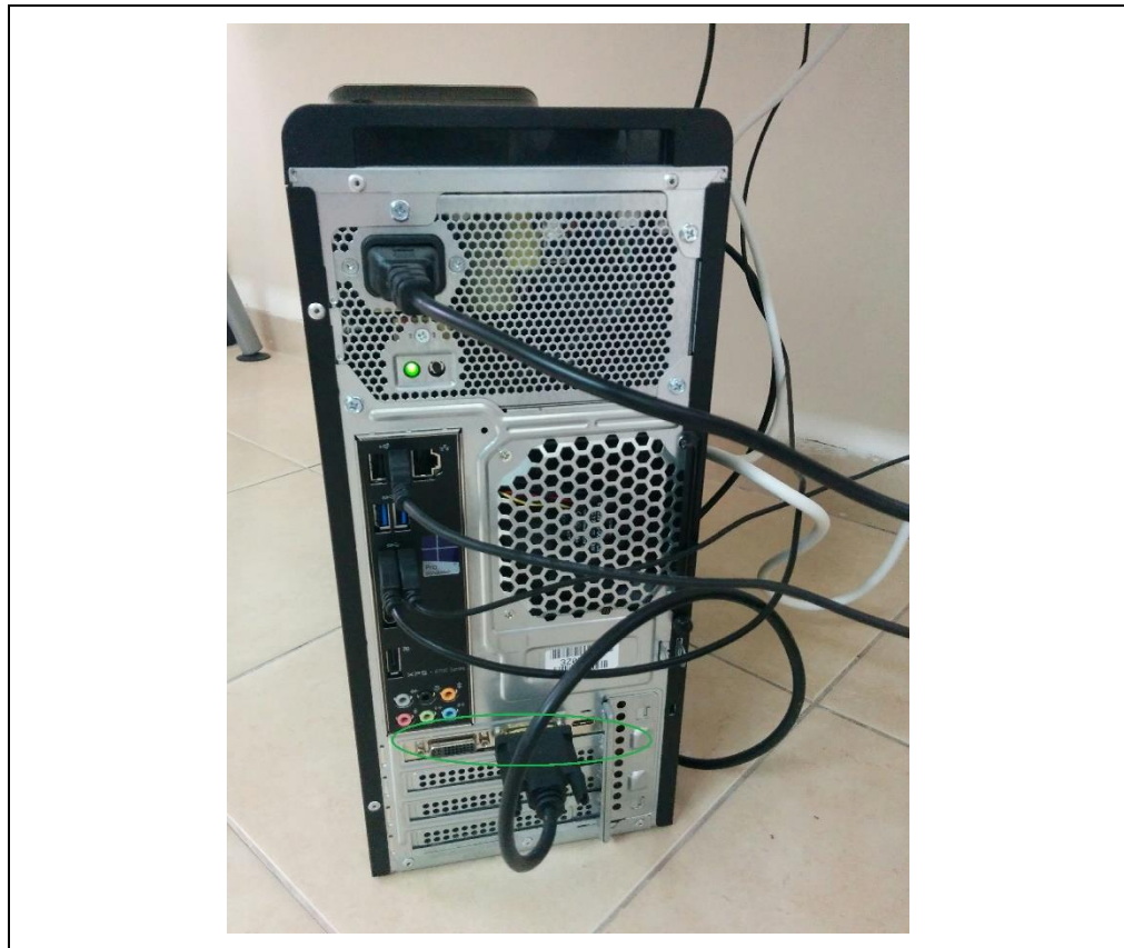
Figure 16: Monitor DVI Connection to PC
