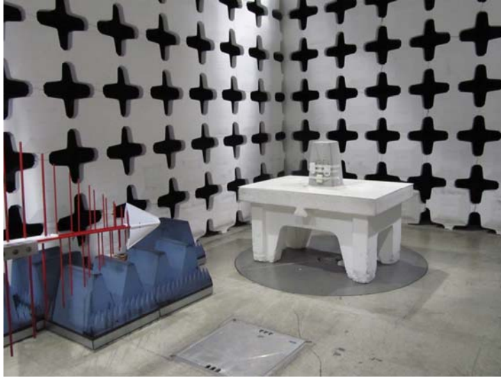
Radiated emissions test set up in 30MHz-1GHz freq. range
