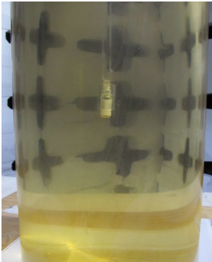
Radiated emissions test set inside human body simulator. Vertical position
