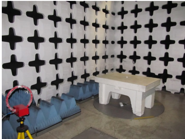
Radiated emissions test set up below 30MHz outside human body simulator.
