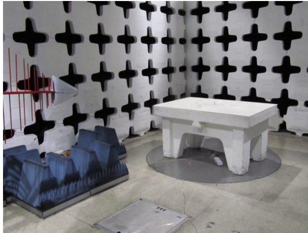
Radiated emissions test set up in 30MHz-1GHz freq. range outside human body simulator.
