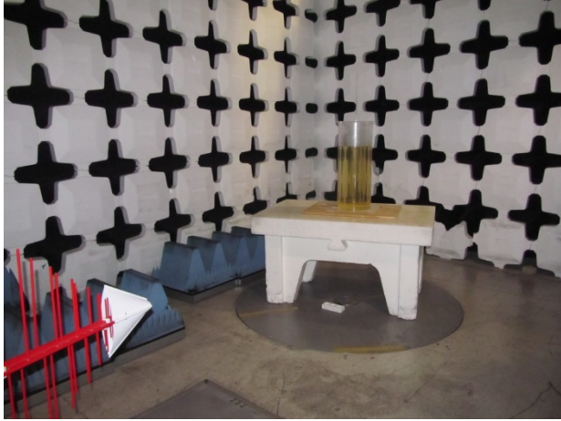
Radiated emissions test set up in 30MHz-1GHz freq. range inside human body simulator.
