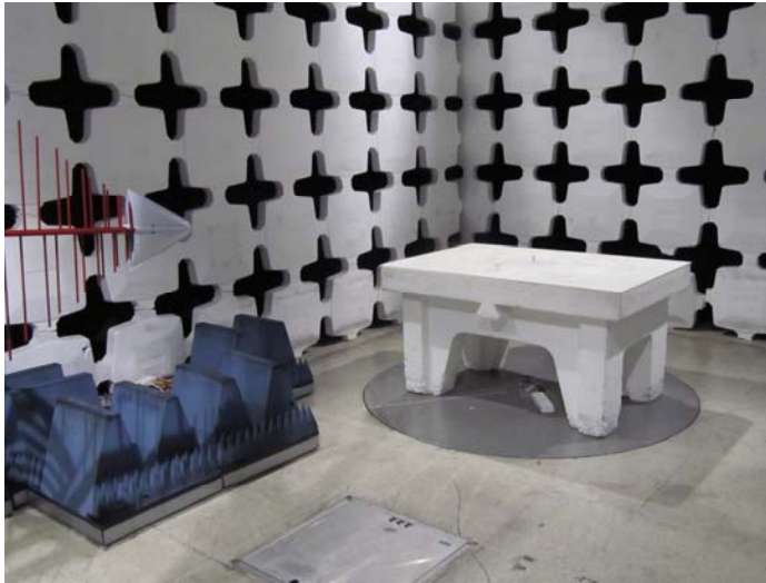
Radiated emissions test set up in 30MHz-1GHz freq. range outside human body simulator.
