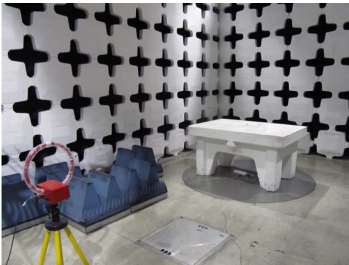
Radiated emissions test set up below 30MHz outside human body simulator.
