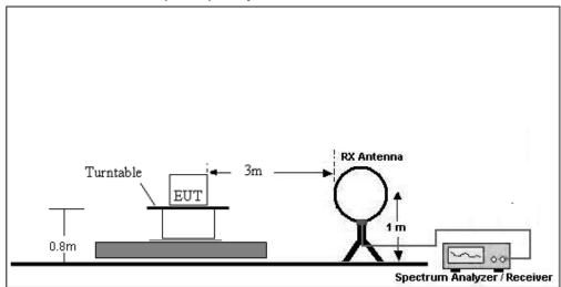
(B) Radiated Emission Test-Up Frequency 30MHz~1GHz
