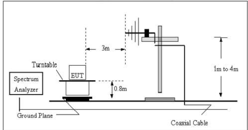
(C) Radiated Emission Test-Up Frequency Above 1GHz
