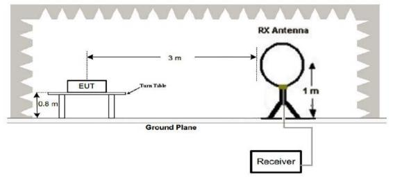
(2) Radiated Emission Test-Up Frequency 30MHz~1GHz
