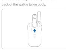
Step 3: Remove the cover of the **Battery** Compartment, and install 4 pieces of AAA until it clicks into place. batteries into it.
