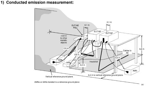
**Note:** The 0.8 m distance specified between EUT/AE/PSU and AMN/AAN, is applicable only to the EUT being measured. If the device is AE then it shall be >0.8 m.
