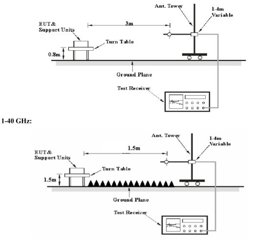
The radiated emission tests were performed in the 3 meters chamber test site, using the setup accordance with the ANSI C63.10-2013. The specification used was FCC 15.209, FCC 15.407 limits.
