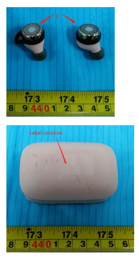
Conclusion: Based on the above description of area A to B, we conclude that the device is unquestionably too small for enabling the FCC certification No. to be printed onto any surface. We therefore request to move the FCC certification No. to the user's manual and charging case.
