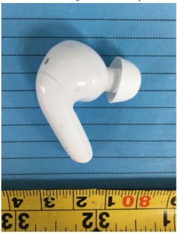
B. Top cover (B): The top cover does not provide enough physical space to fit the printing of the FCC certification No. according to below reference picture.
