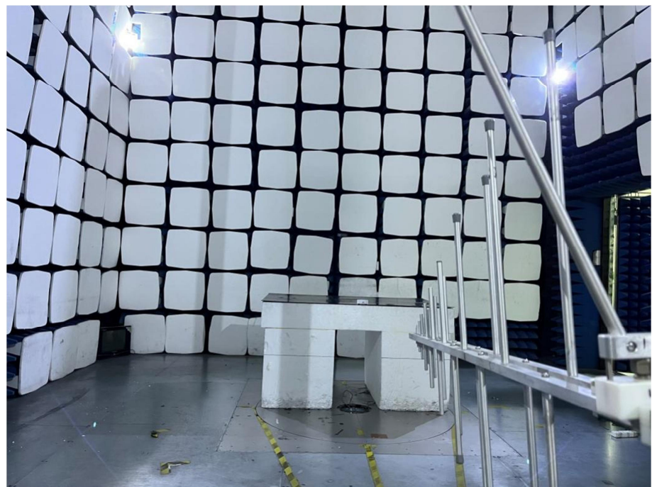
Radiation Emission Test Setup (30MHz to 1GHz)
