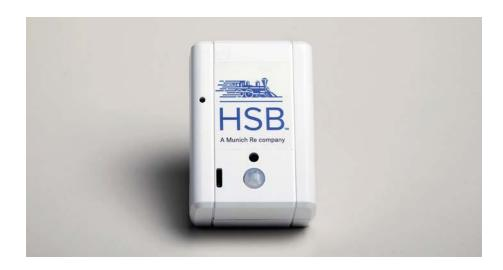
The Meshify Ambient Temperature Sensor is designed for indoor residential or commercial applications to detect multiple environmental conditions. The sensor is not intended for industrial or heavy duty use. The sensor is powered by a two replaceable AA batteries, eliminating the need for an electrical outlet.
