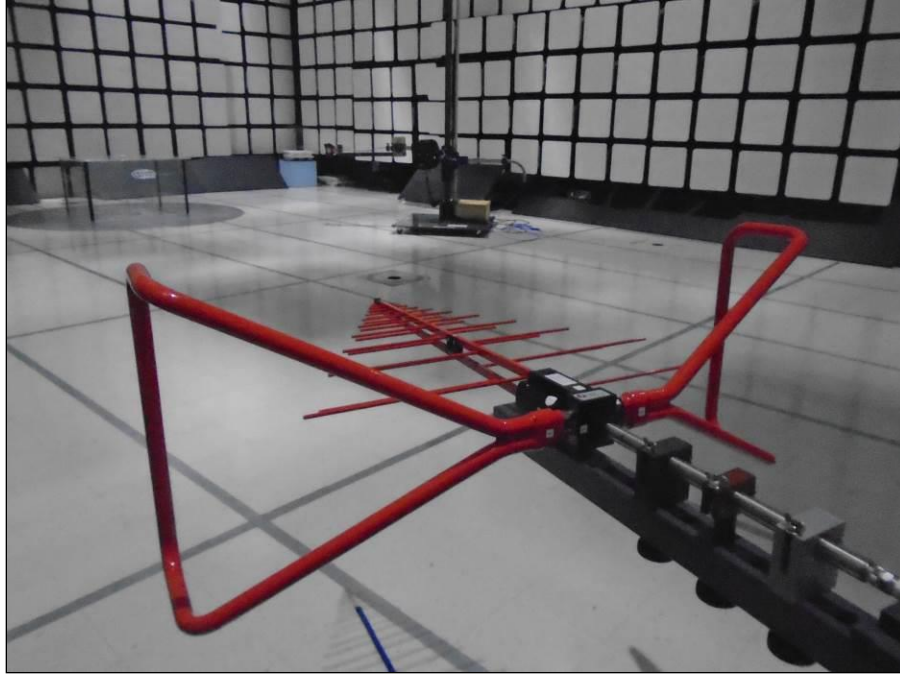
Photograph 5. Radiated Spurious Emissions, 30-1000 MHz Antenna
