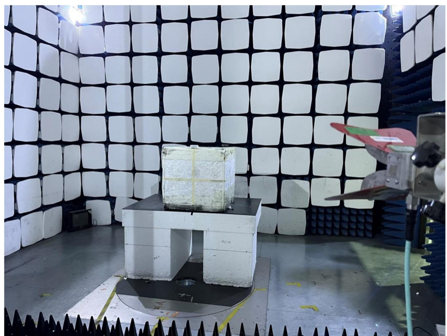
Radiation Emission Test Setup (1GHz to 18GHz)
