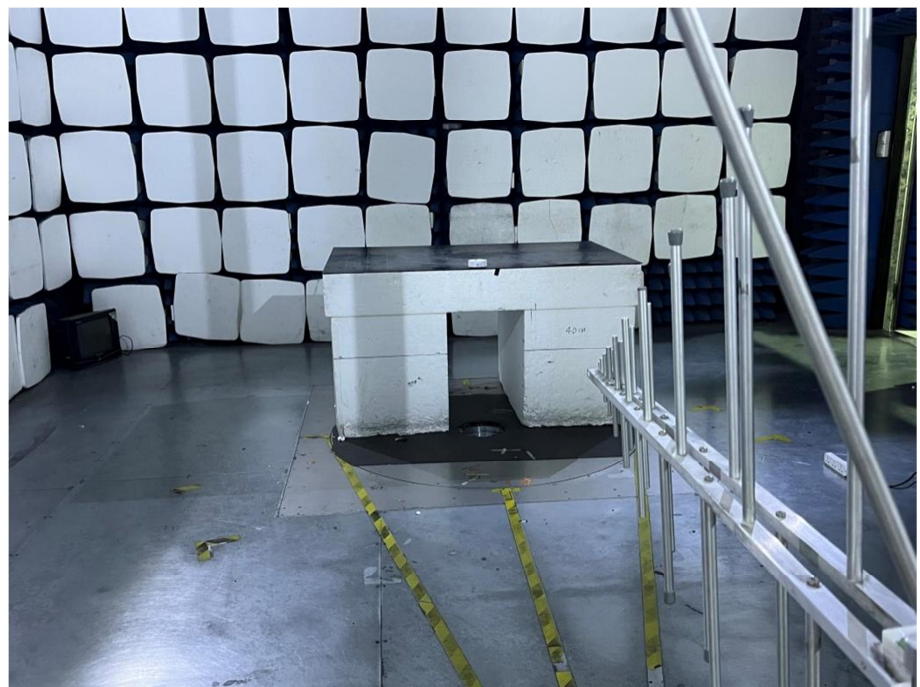
Radiation Emission Test Setup (30MHz to 1GHz)
