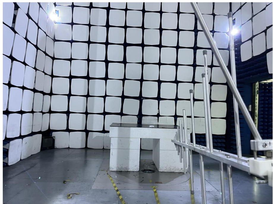
Radiation Emission Test Setup (30MHz to 1GHz)
