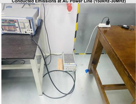
Conducted Emissions at AC Power Line (150kHz-30MHz)
