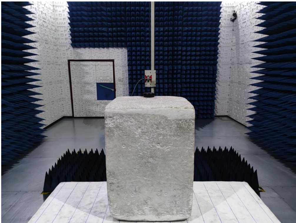
RADIATED EMISSION TEST SETUP ABOVE 1GHZ
