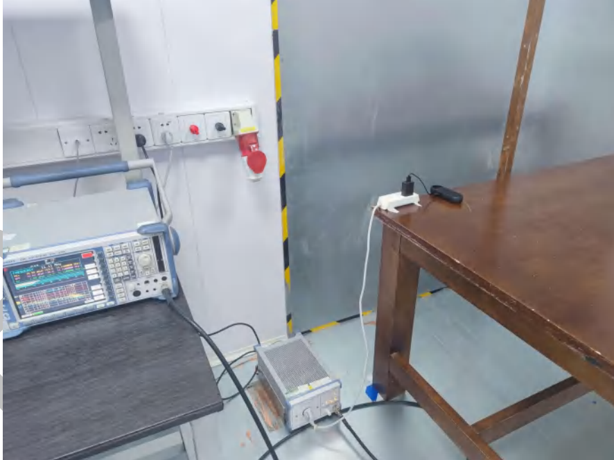
Conducted Emissions at AC Power Line (150kHz-30MHz)
