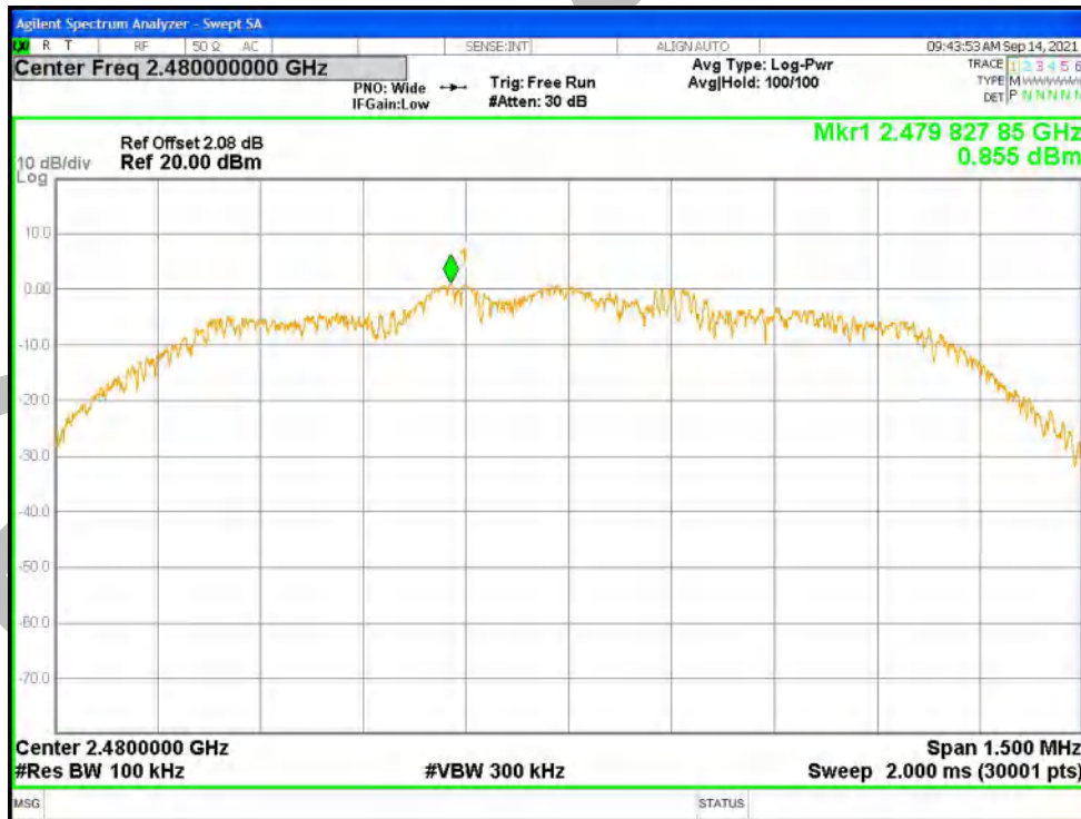
Tx. Spurious NVNT 2-DH1 2480MHz Ant1 Emission
