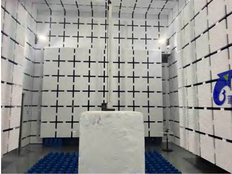
Conducted Emissions at AC Power Line (150kHz-30MHz)
