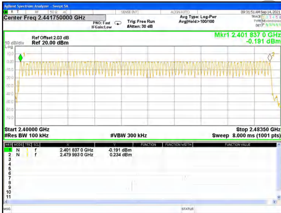
Hopping No. NVNT 2-DH1 2441MHz Ant1
