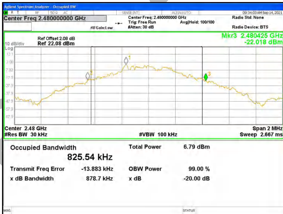
-20dB Bandwidth NVNT 2-DH1 2402MHz Ant1
