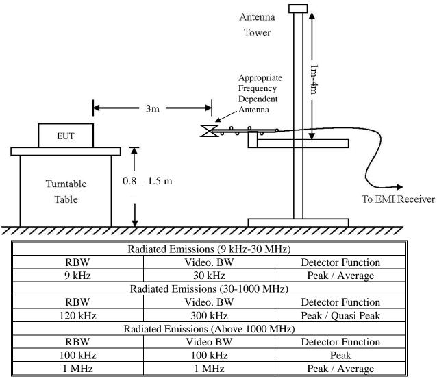
Diagram 2 Test arrangement for radiated emissions tested on Open Area Test Site (OATS)
