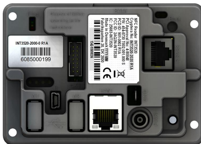
Figure 5 – Back-side view w/ connectors etc.
