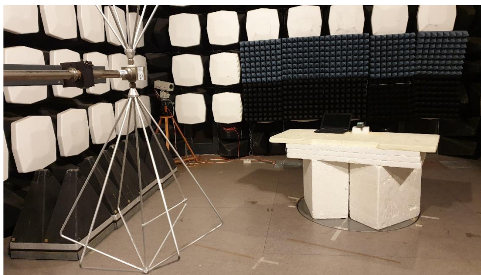
Photo 3. Radiated emission test setup for 30 - 200 MHz.
