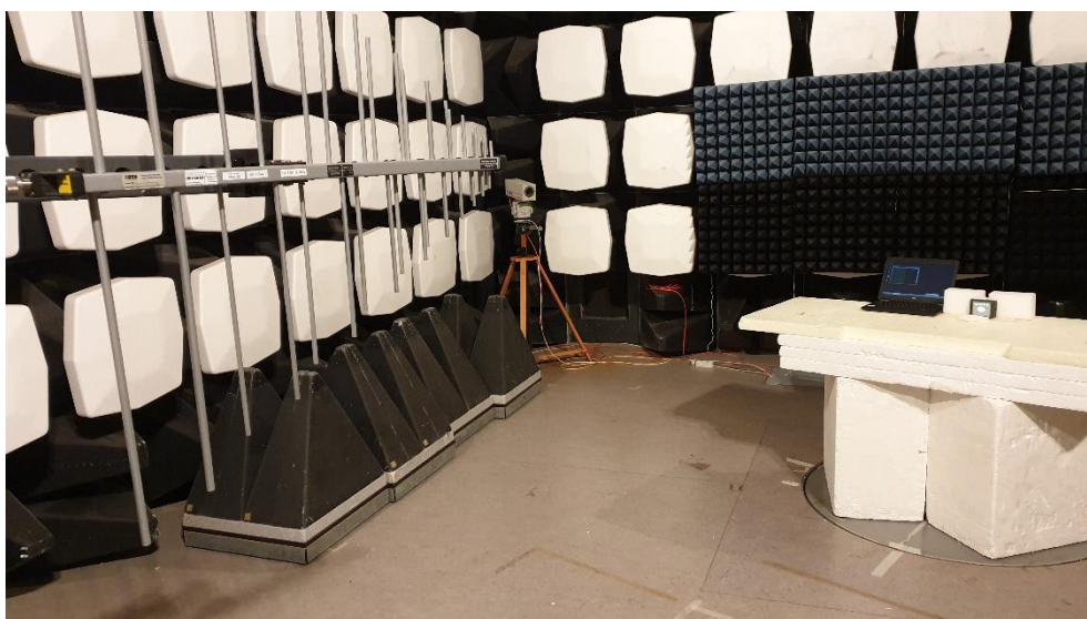
Photo 4. Radiated emission test setup for 200 - 1000 MHz.
