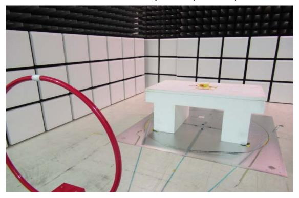
Radiated Emission Setup Photos (30MHz~1GHz)
