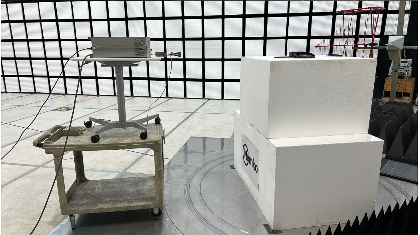
Radiated Emissions, 1 GHz to 26.5 GHz
