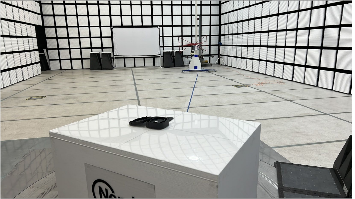
Radiated Emissions, 30 MHz to 1 GHz
