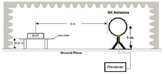
(2) Radiated Emission Test-Up Frequency 30MHz~1GHz
