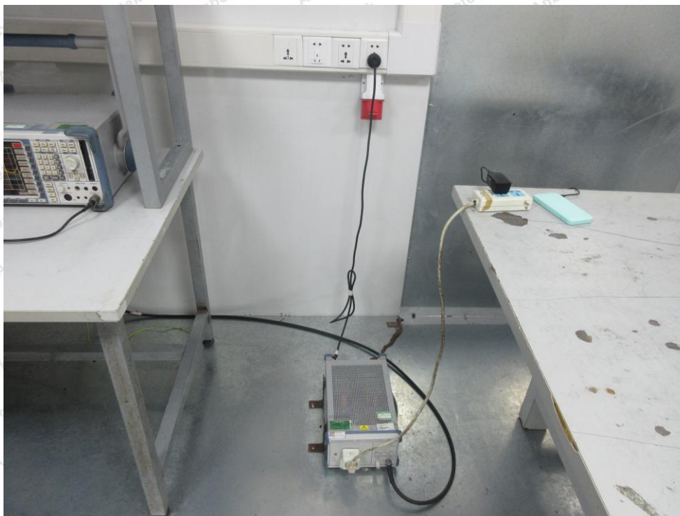
Photo of Conducted Emission Measurement
