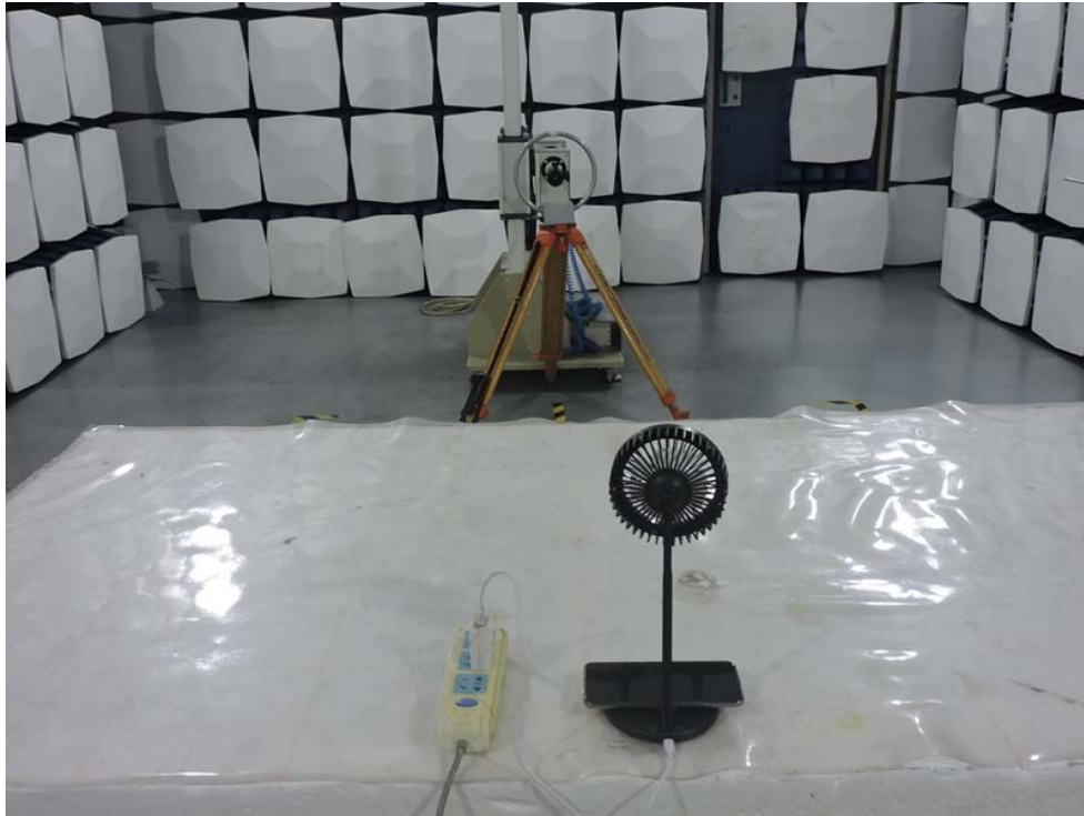
Radiated Emission Test Setup:
