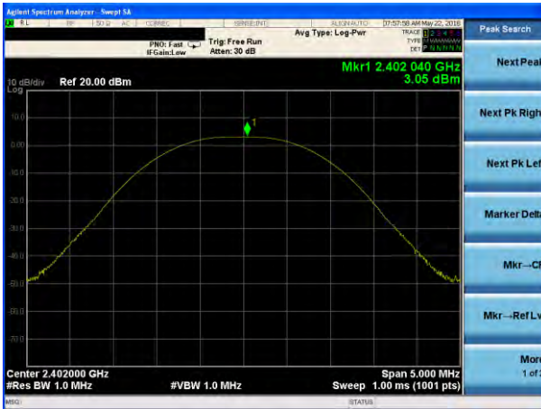
Peak output Power plot on channel 39 (1Mbps)
