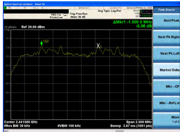
(2Mbps) Channel Separation plot on channel 39-40
