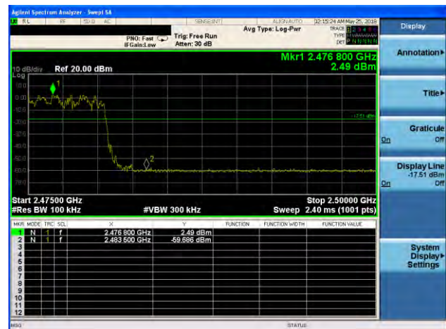
\pi /4-DQPSK: Band Edge-High Channel (Hopping Mode)
