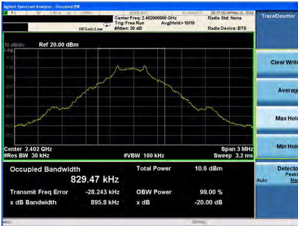
20dB Bandwidth plot on channel 39 (1Mbps)
