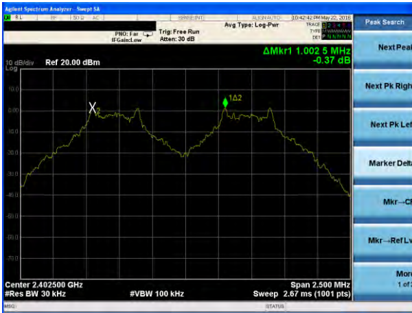
(1Mbps) Channel Separation plot on channel 39-40
