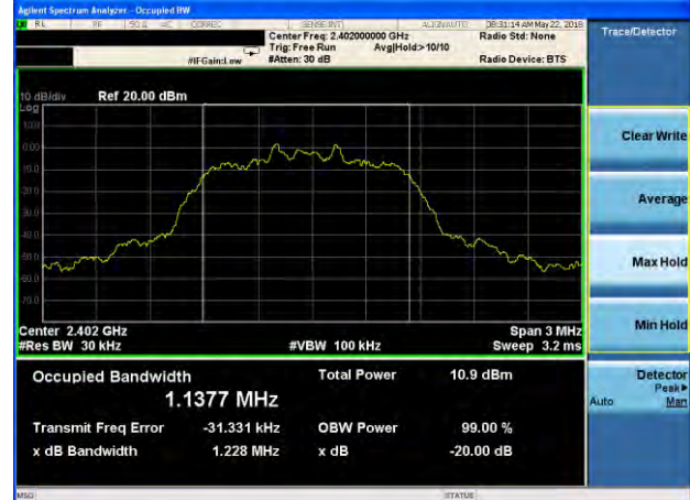
20dB Bandwidth plot on channel 39 (2Mbps)
