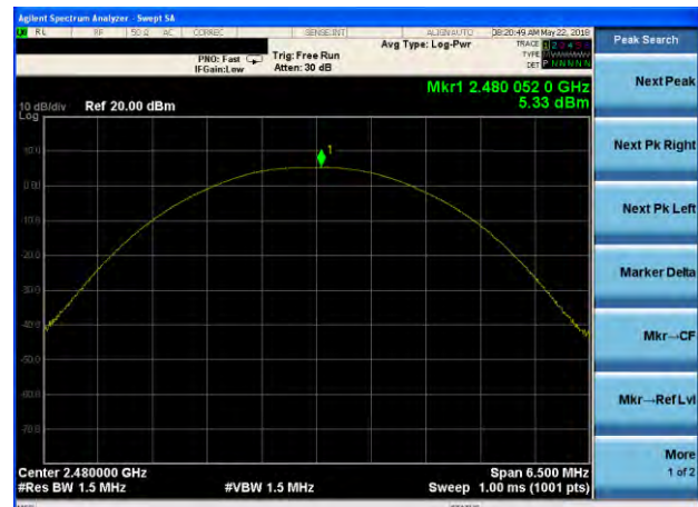
Peak output Power plot on channel 78 (2Mbps)
