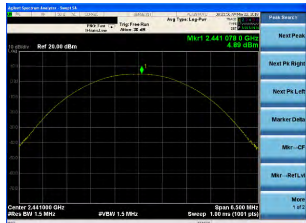
Peak output Power plot on channel 39 (2Mbps)
