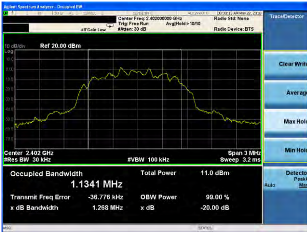
20dB Bandwidth plot on channel 39 (3Mbps)
