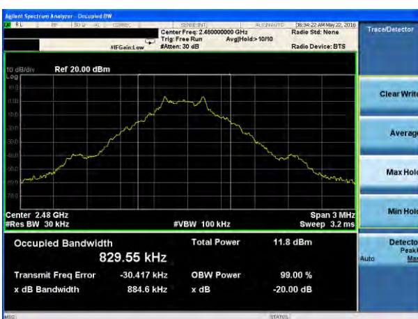
20dB Bandwidth plot on channel 78 (1Mbps)
