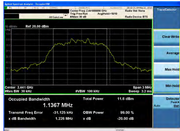
20dB Bandwidth plot on channel 78 (2Mbps)
