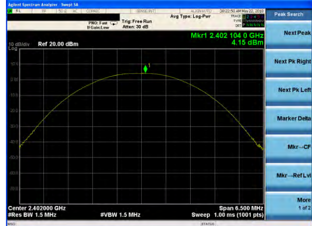
Peak output Power plot on channel 39 (2Mbps)
