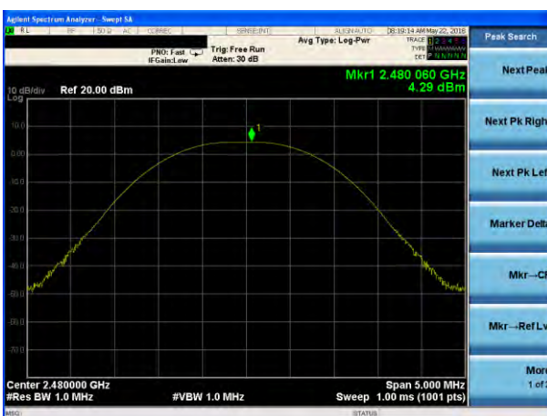
Peak output Power plot on channel 78 (1Mbps)
