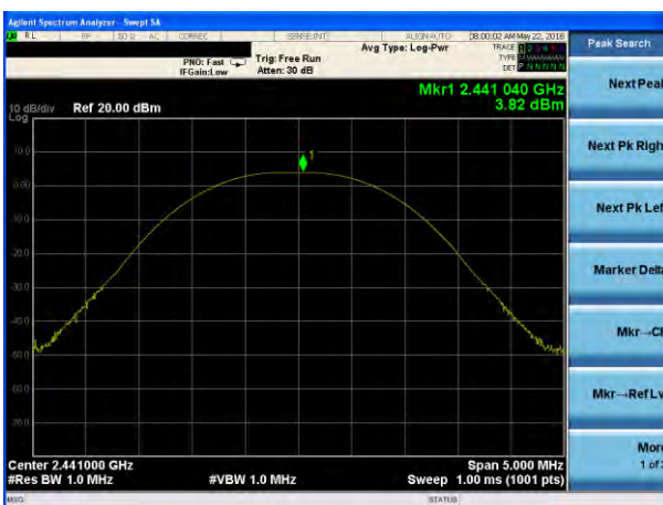
Peak output Power plot on channel 39 (1Mbps)
