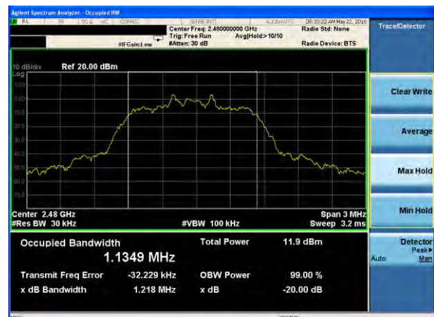
20dB Bandwidth plot on channel 78 (2Mbps)
