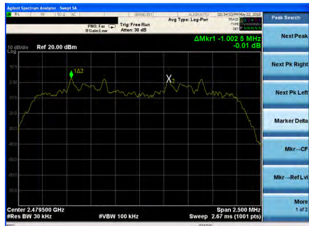
(2Mbps) Channel Separation plot on channel 77-78
