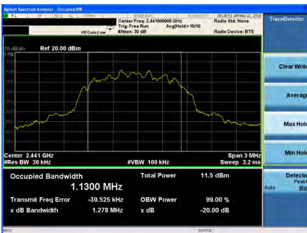
20dB Bandwidth plot on channel 39 (3Mbps)
