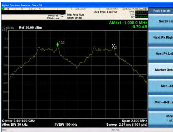
(1Mbps) Channel Separation plot on channel 39-40
