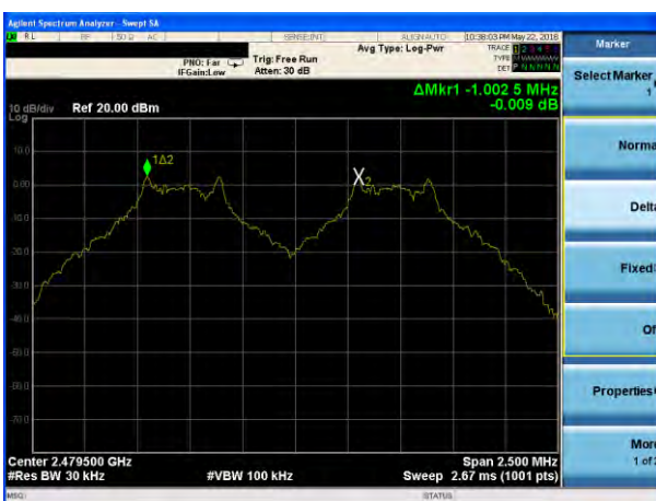
(1Mbps) Channel Separation plot on channel 77-78
