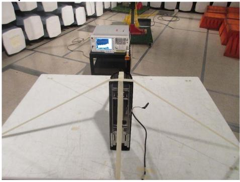
1.11 Radiated Spurious Emission 60-90 GHz Front View
