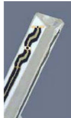
Figure 2.3 Probe Thick-Film Technique
