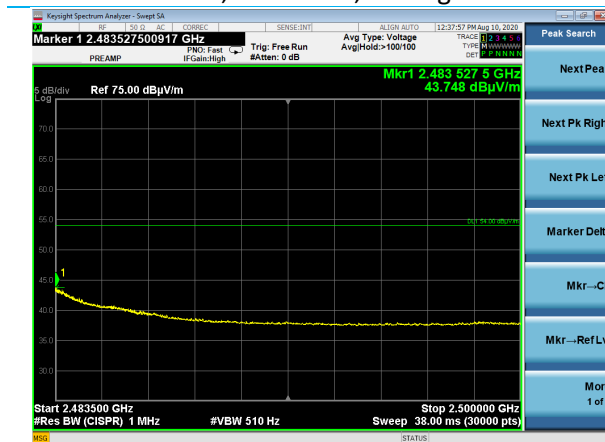
2483.5-2500 MHz, Vertical Antenna, Side EUT BLE, Channel 39, Average
